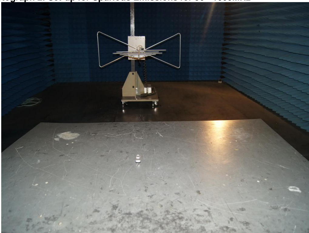
Photograph 2: Set-up for Spurious Emissions for 30 - 1000MHz
