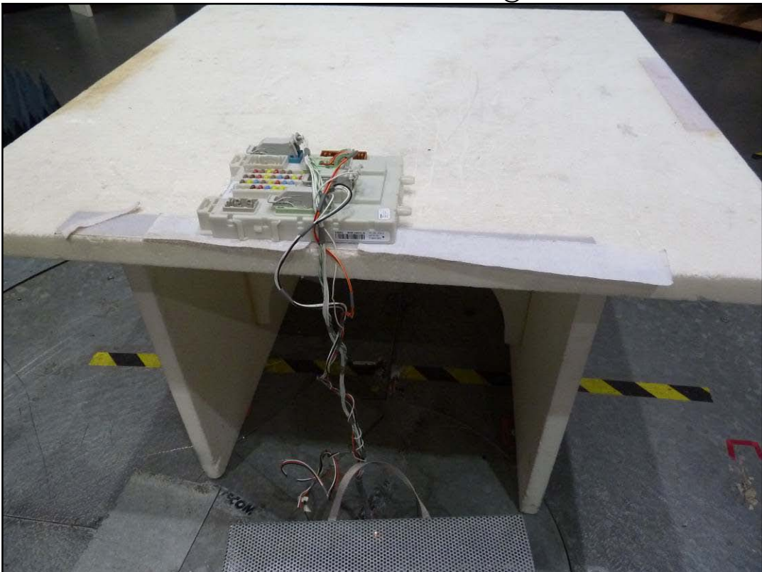
Photo 2: radiated emission < 1GHz @ 10m
