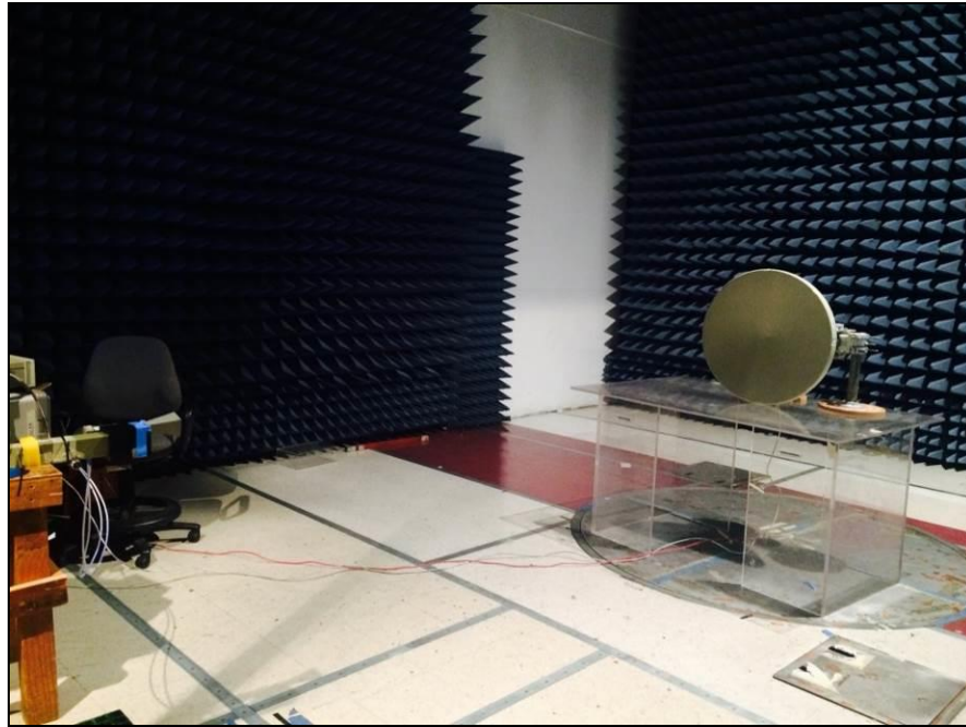
Photograph 6. Radiated Spurious Emissions, Test Setup, Above 18-40GHz
