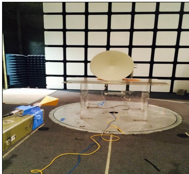
Photograph 7. Radiated Spurious Emissions, Test Setup, Above 40 GHz
