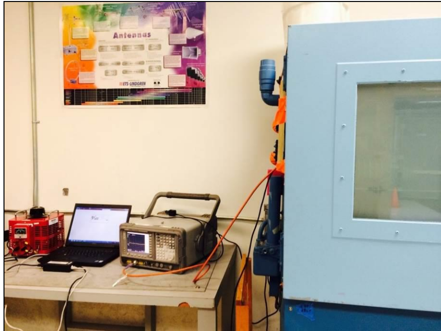
Photograph 2. Frequency Tolerance, Test Setup
