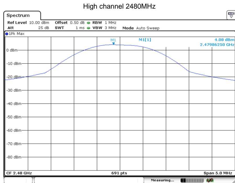
Bluetooth Mode  $\pi/4$ -DQPSK modulation Test Result
