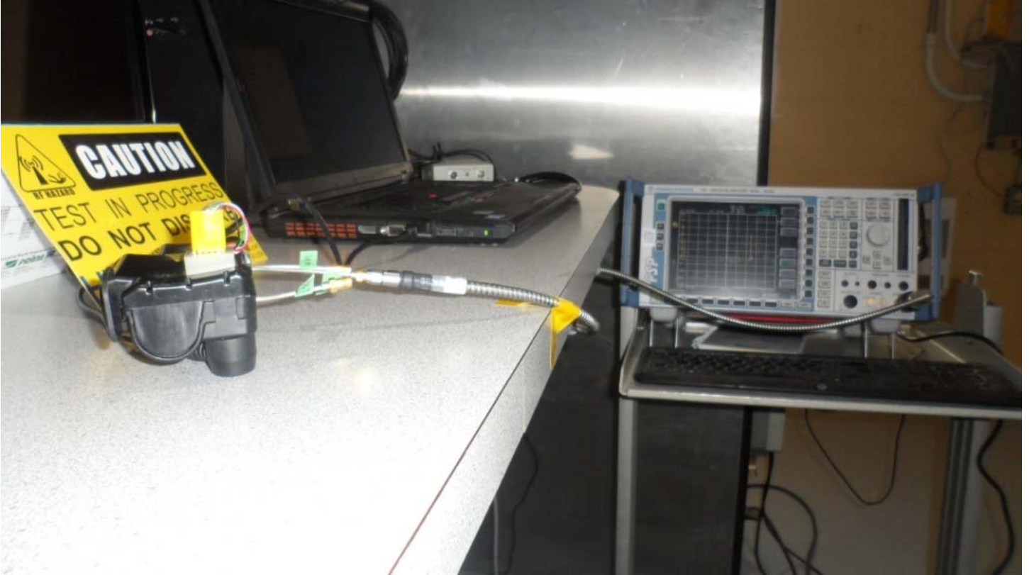
Figure E21.3 – Setup Photo – Conducted Measurements
