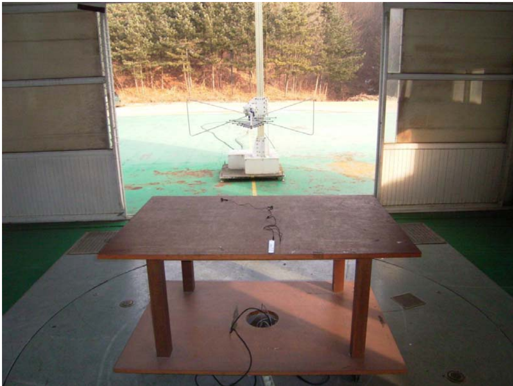
Radiated Emissions(FM receiving mode)-Rear View
