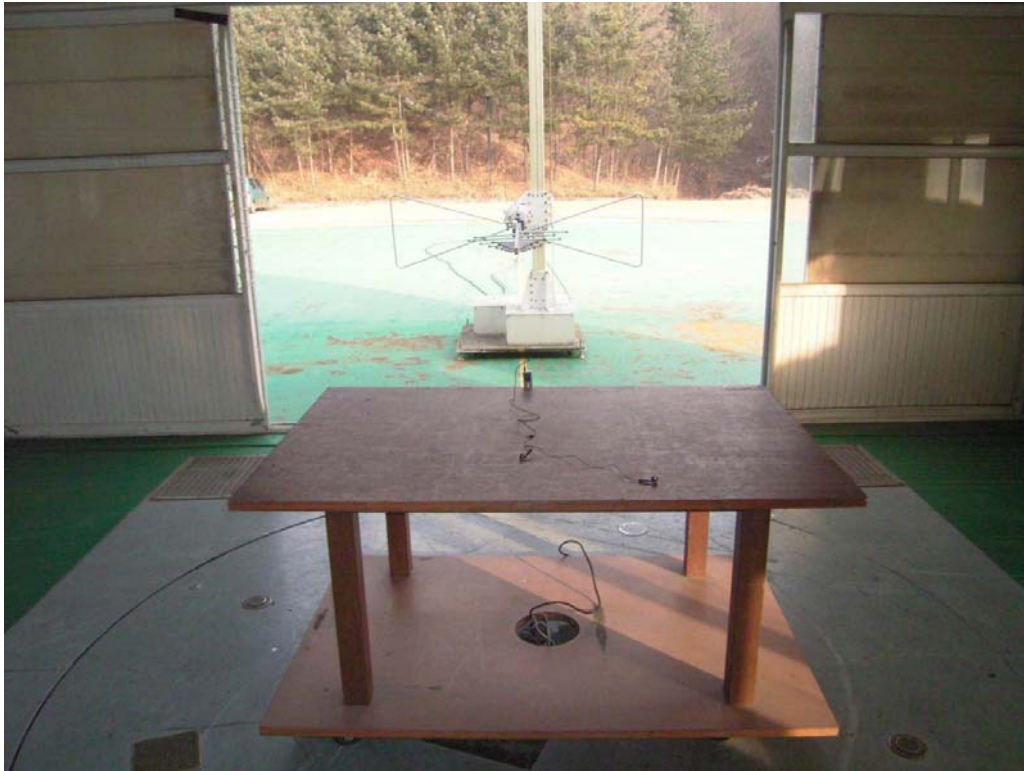
Radiated Emissions(FM receiving mode)-Front View
