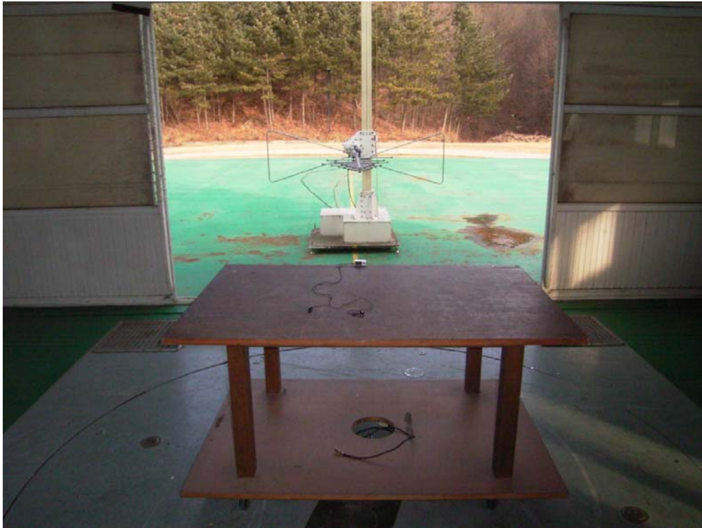
Radiated Emissions(FM receiving mode)-Front View
