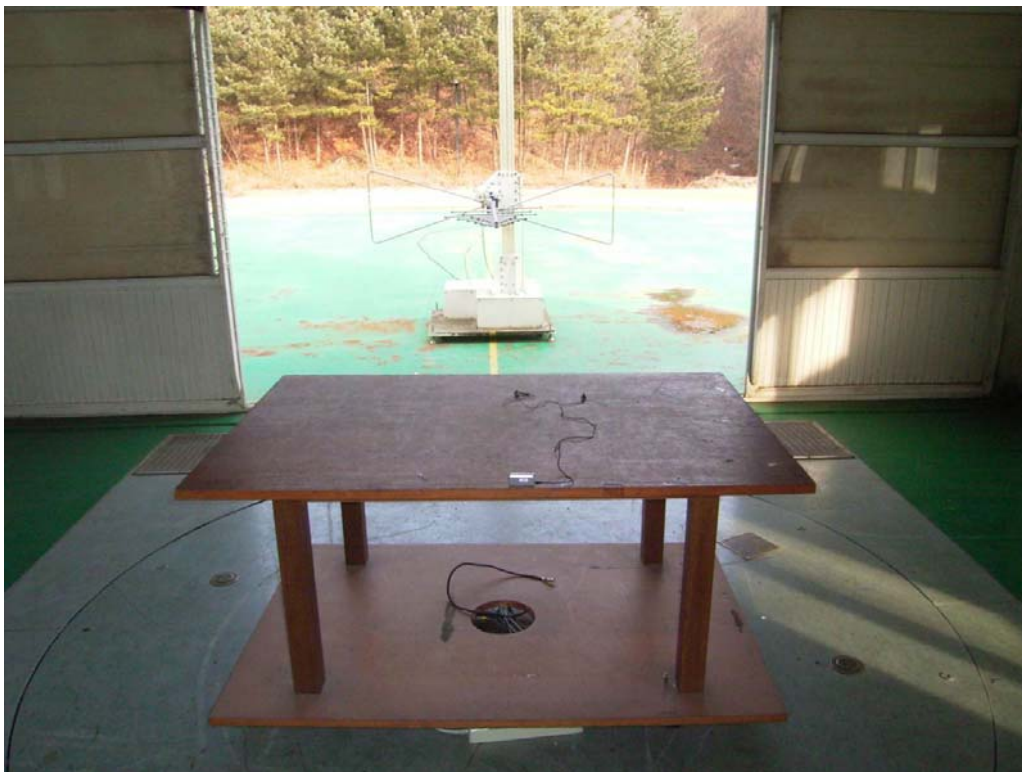
Radiated Emissions(FM receiving mode)-Rear View
