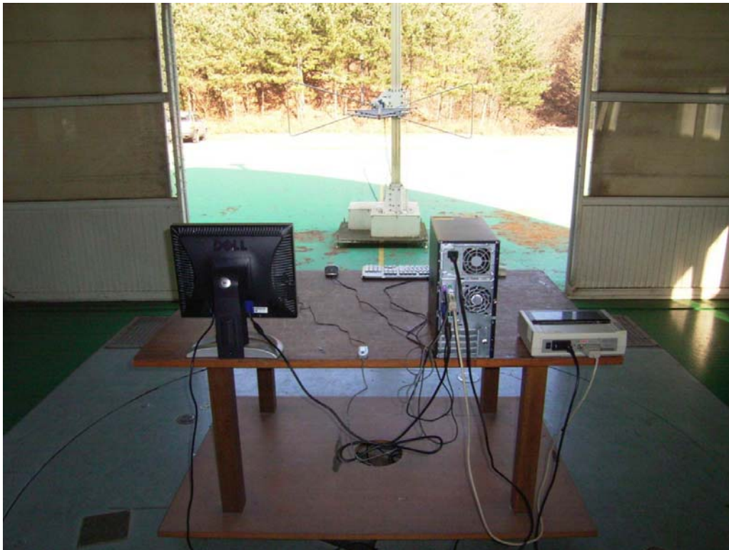
Radiated Emissions(File up/download mode) - Rear View
