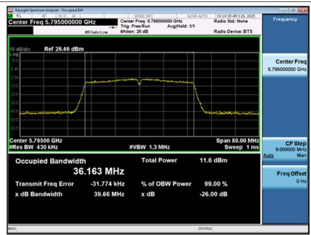
802.11ac(VHT80) 26 dB Bandwidth (CH 155)
