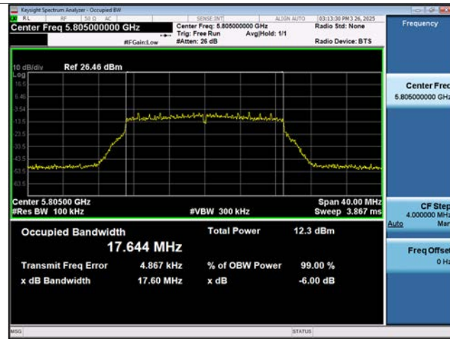
802.11ac(VHT40) 6 dB Bandwidth (CH 151)
