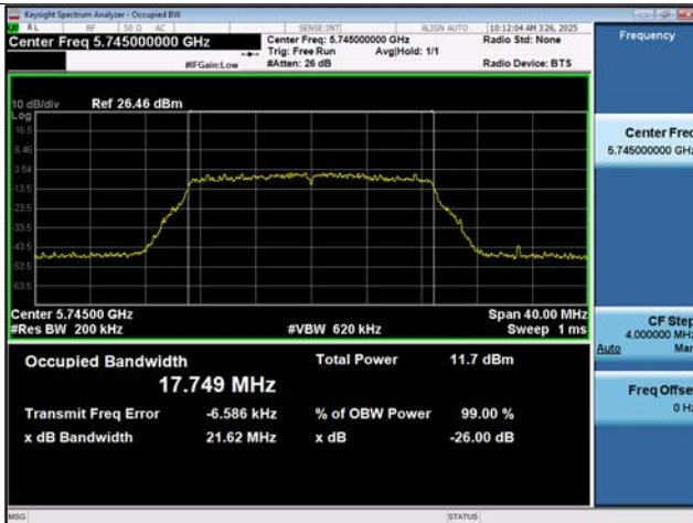
802.11ac(VHT40) 26 dB Bandwidth (CH 151)
