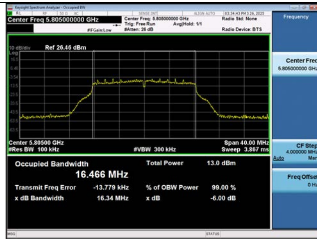
802.11ac(VHT20) 6 dB Bandwidth (CH 161)
