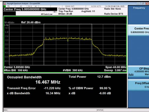
802.11ac(VHT20) 6 dB Bandwidth (CH 157)
