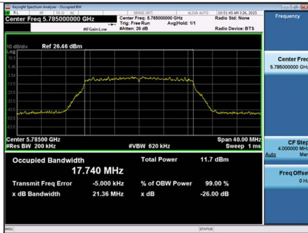
802.11ac(VHT40) 26 dB Bandwidth (CH 159)
