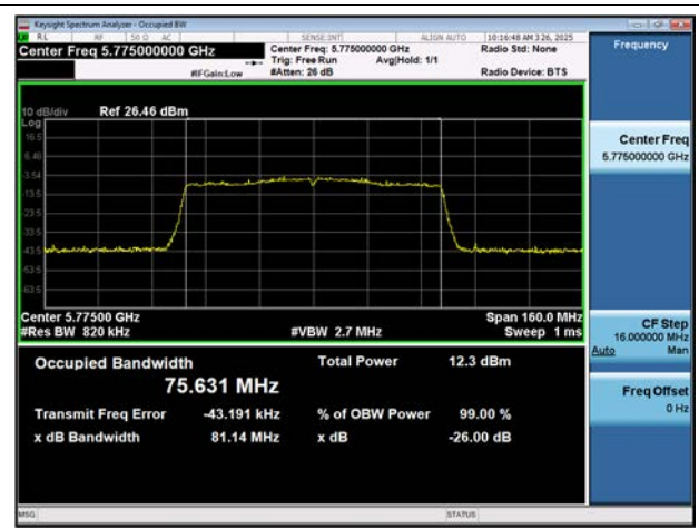
802.11ac(VHT80) 26 dB Bandwidth (CH 155)
