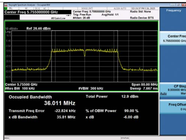
802.11ac(VHT40) 6 dB Bandwidth (CH 151)
