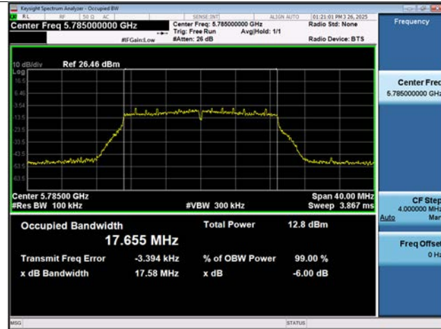
802.11ac(VHT40) 6 dB Bandwidth (CH 151)
