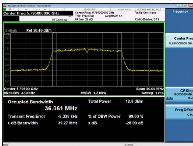
802.11ac(VHT40) 26 dB Bandwidth (CH 159)
