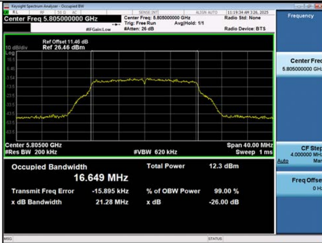
802.11ac(VHT20) 26 dB Bandwidth (CH 149)
