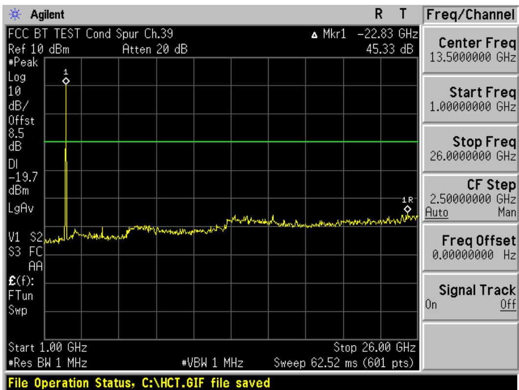
Test Plots (8DPSK) - 1 GHz - 26 GHz (RBW:1 MHz, VBW: 1 MHz)
