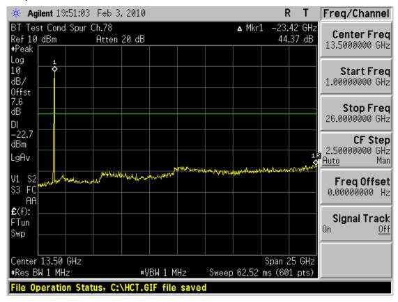
Test Plots(8DPSK) -1 GHz ~ 26 GHz (RBW: 1 MHz, VBW: 1 MHz) ( Low CH )
