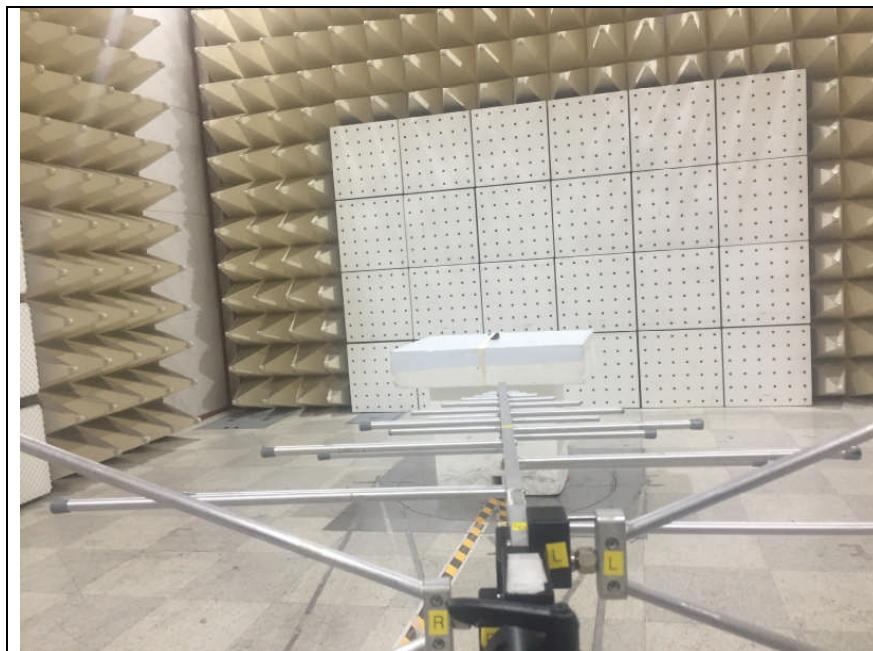
**3. Photo of Radiated Spurious Emission Test (Above 1 GHz)**
