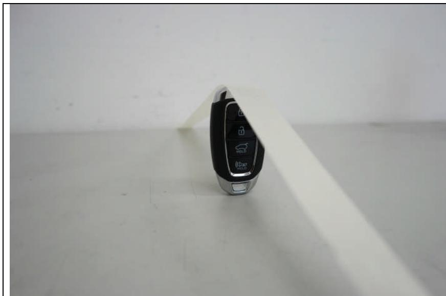
**2. Photos of Radiated Spurious Emission Test (Below 1 GHz)**
