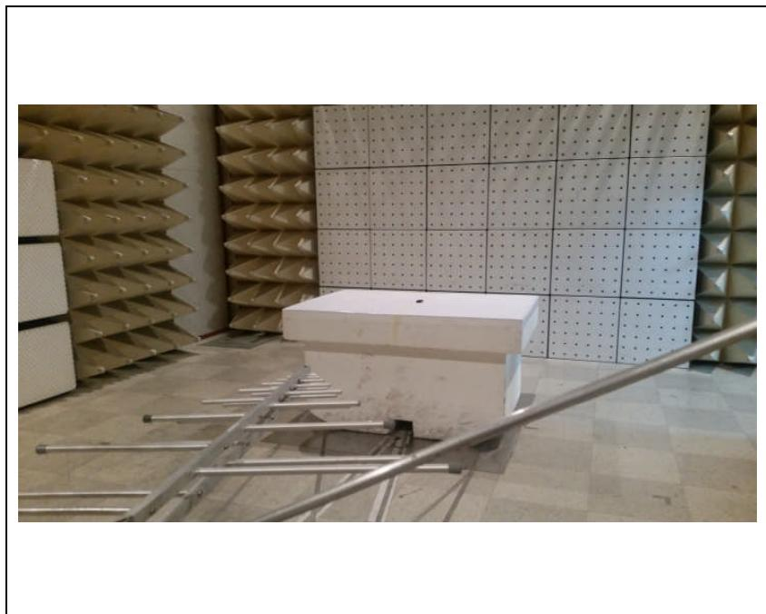
**D. Photo of Test setup (1 GHz ~ 4.5 GHz)**
