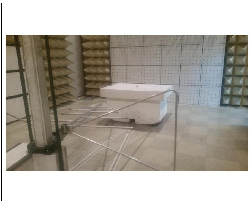
**B. Photo of Radiated Spurious Emission Test (Above 1GHz)**
