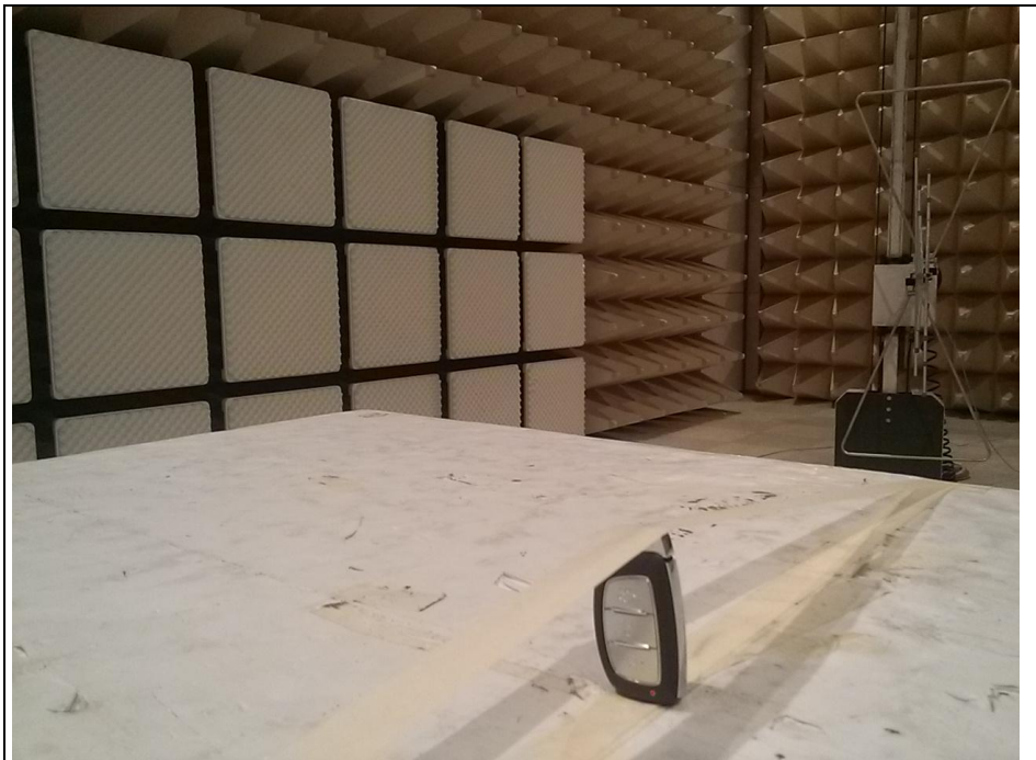
Photo of Test Set up (30 MHz ~ 1 GHz)
