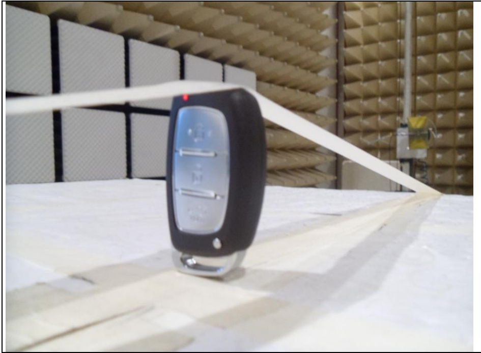
Photo of Test Set up (Above 1 GHz)
