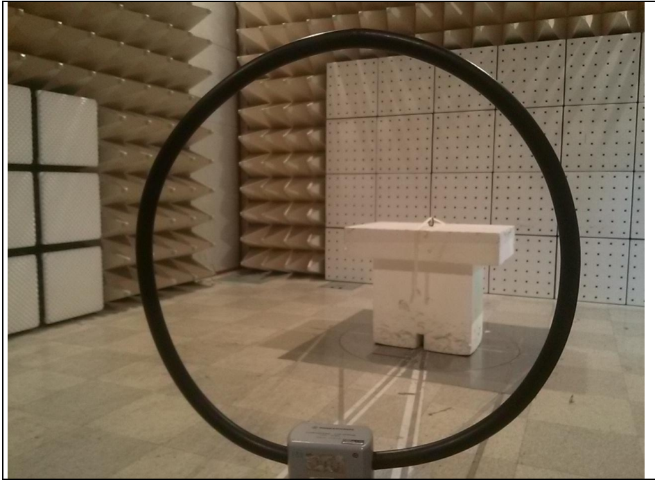
Photo of Test Set up (30 MHz ~ 1 GHz)
