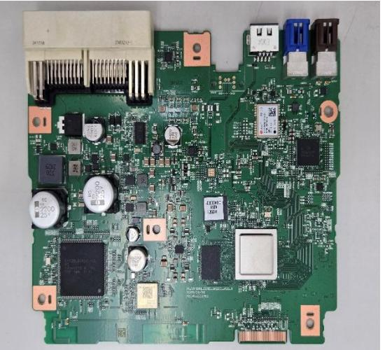
A photograph of a green printed circuit board (PCB) for a system without a camera. The board is densely populated with components, including a central processor, memory chips, and various connectors. Orange and white heat sinks are attached to the board, notably on the left side and near the top center. The board is mounted on a light-colored plastic frame.                             |
