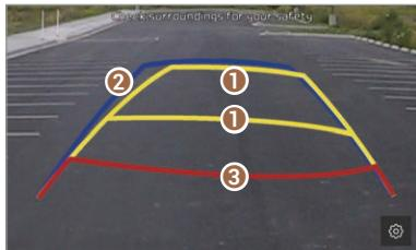
① Driving direction lines (yellow). These lines show the directions of the vehicle according to the steering angle.
