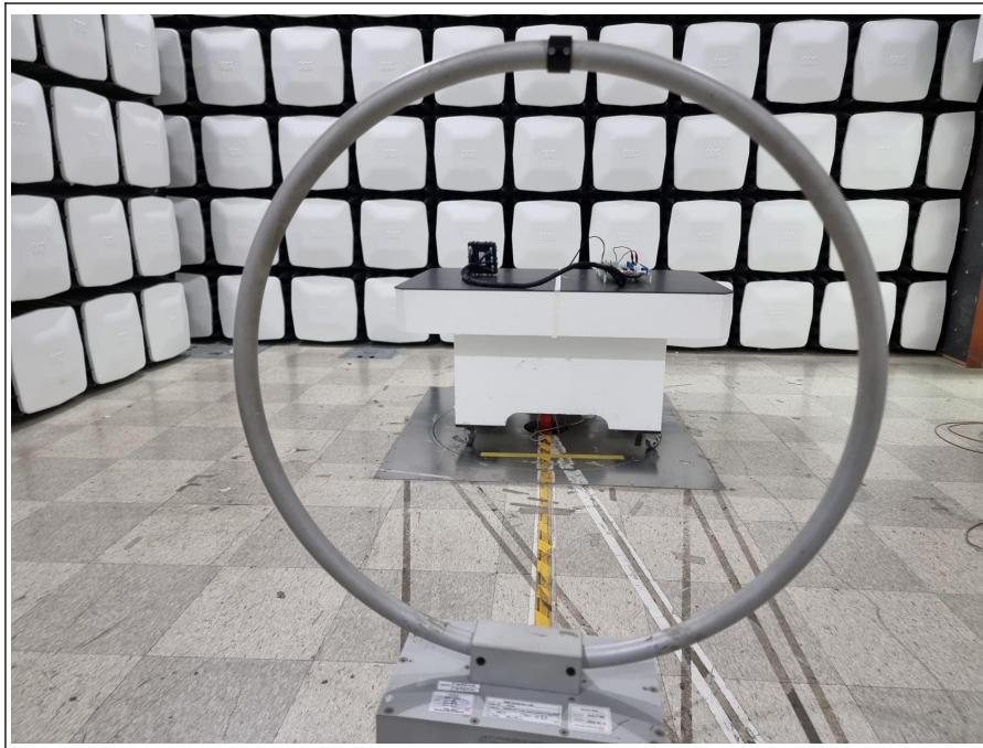
**2. Photo of Radiated Spurious Emission Test (30 GHz ~ 1 000 GHz)**
