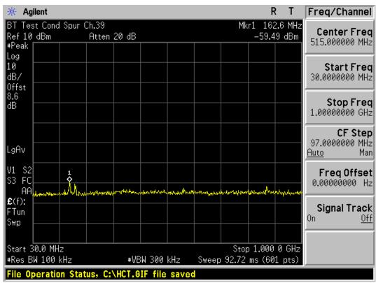
Test Plots (8DPSK) - 30 MHz - 1 GHz (RBW:100 kHz, VBW: 300 kHz) Spurious Emission (High-CH)
