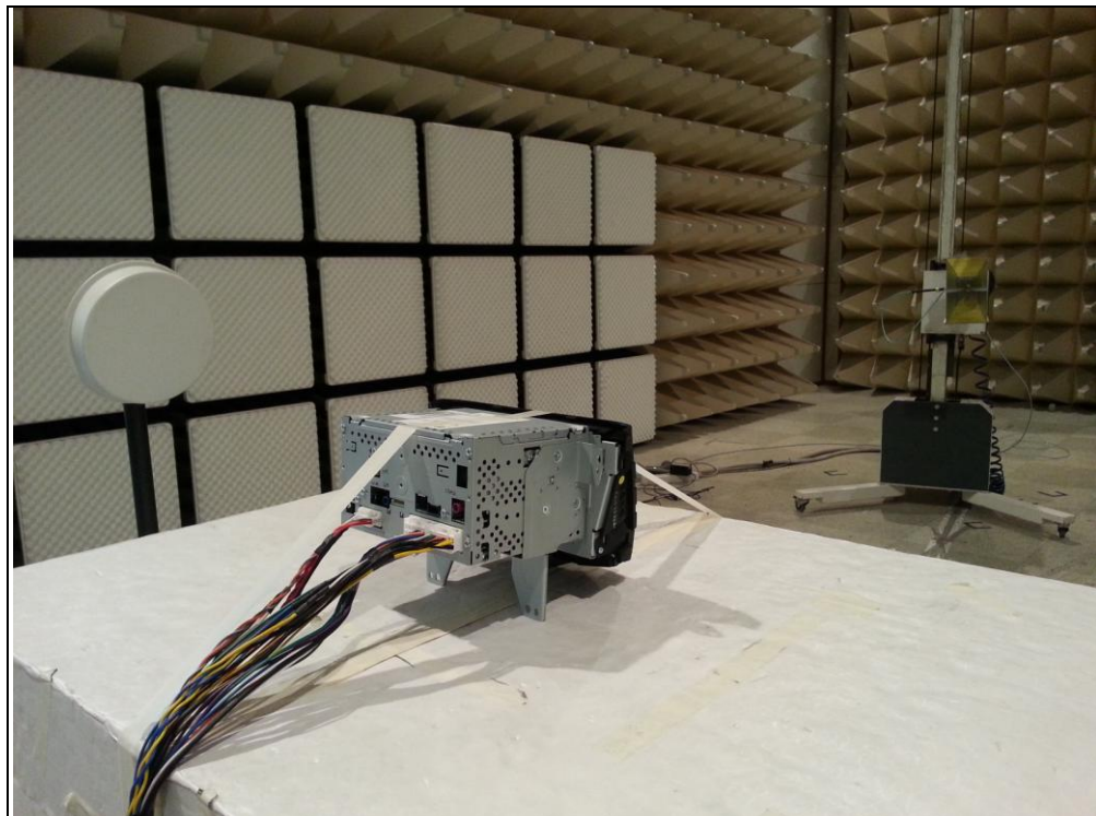
Photo of Field Strength & Spurious Emission Test(BT)
