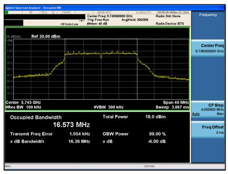
6 dB Bandwidth Test Mode: 802.11a & Ch.157
