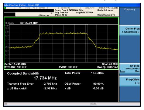
6 dB Bandwidth Test Mode: 802.11n(HT20) & Ch.157
