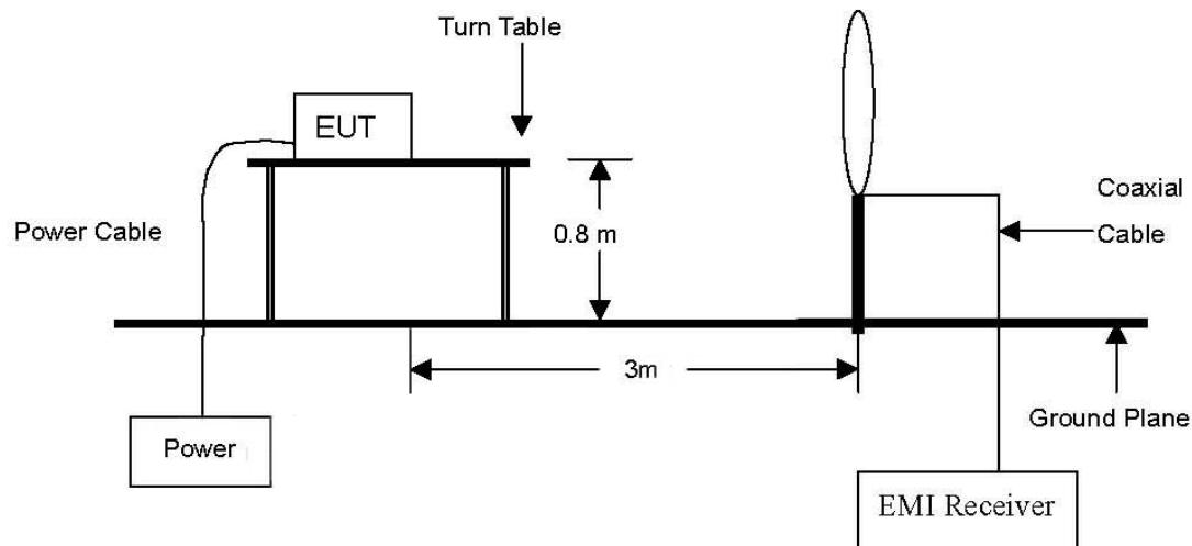
The diagram below shows the test setup that is utilized to make the measurements for emission from 30 MHz to 1 GHz.
