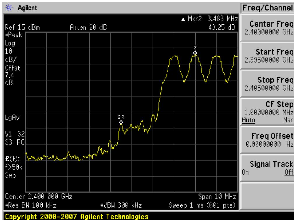
Test Plots with hopping (GFSK)
