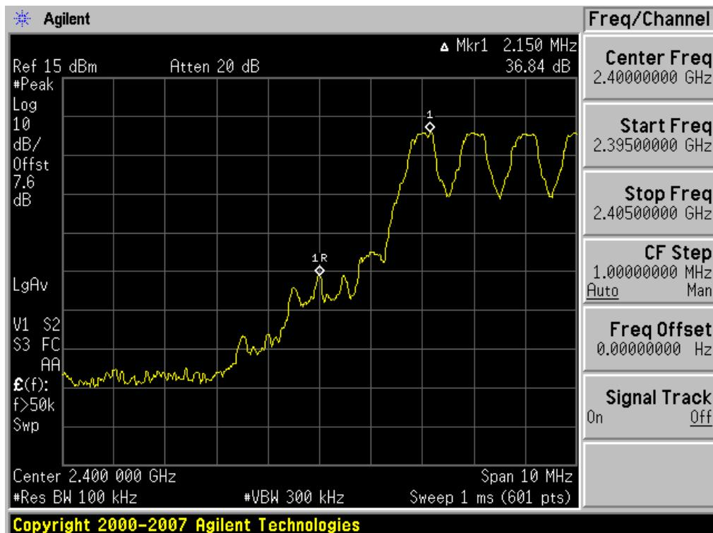
Test Plots with hopping (GFSK)
