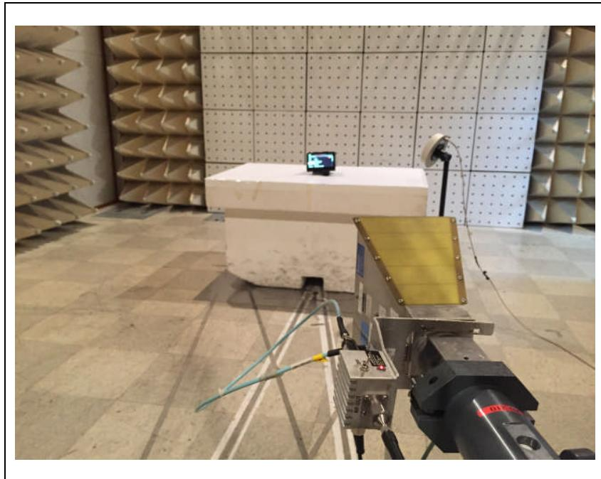
**2.WLAN****A. Photo of Radiated Spurious Emission Test (Below 1 GHz)**
