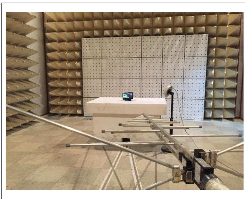
**B. Photo of Radiated Spurious Emission Test (Above 1 GHz)**
