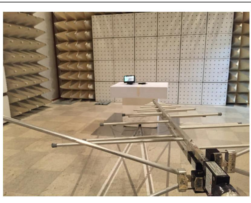
**B. Photo of Radiated Spurious Emission Test (Above 1 GHz)**
