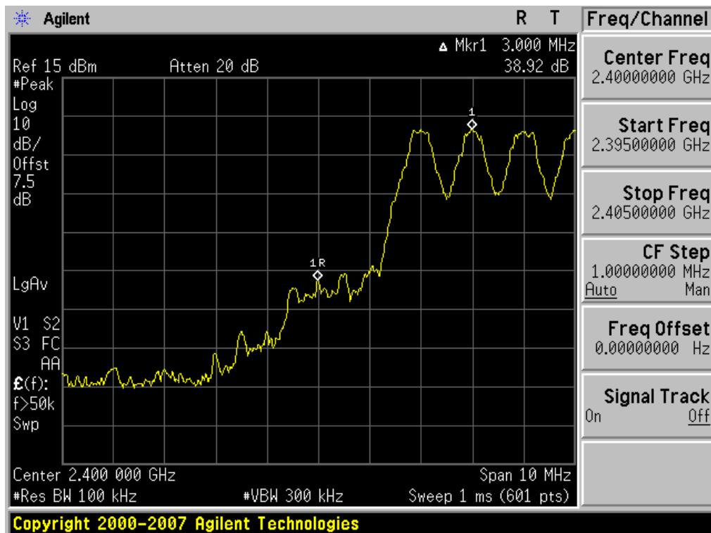
Test Plots with hopping (GFSK)
