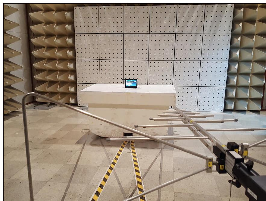
**3. Photo of Radiated Spurious Emission Test (Above 1 GHz)**
