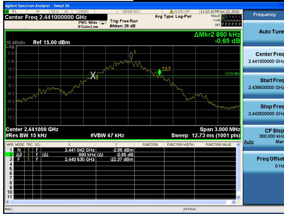
**20 dB Bandwidth****Highest Channel & Modulation : GFSK**
