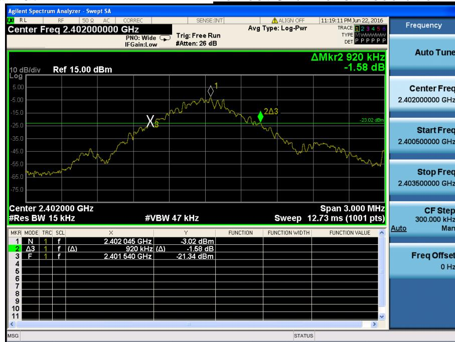
**20 dB Bandwidth****Middle Channel & Modulation : GFSK**
