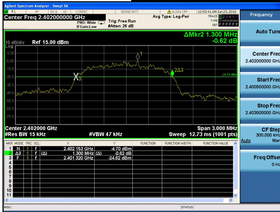
**20 dB Bandwidth****Middle Channel & Modulation : 8DPSK**
