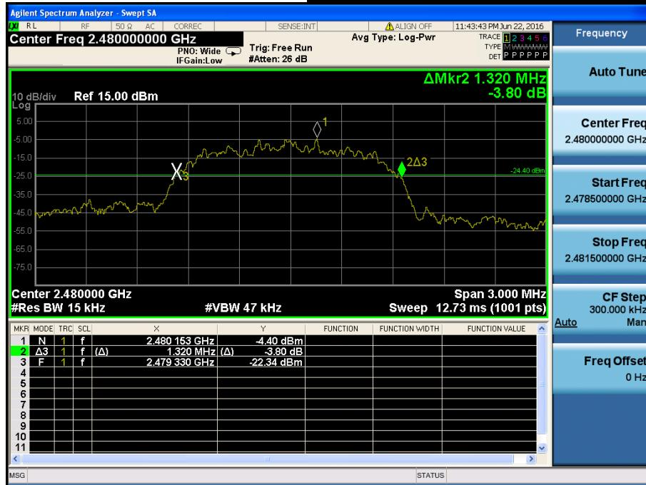
**20 dB Bandwidth****Lowest Channel & Modulation : 8DPSK**
