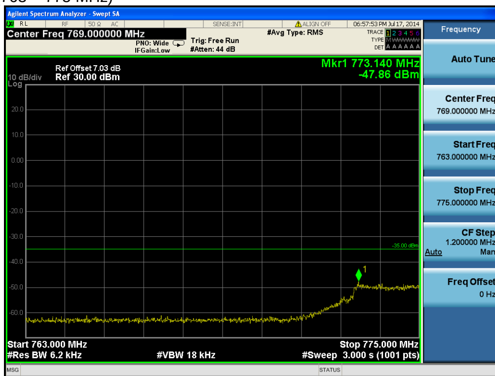
LTE Band 13 / 10MHz / QPSK - RB Offset/Size (0/25)
