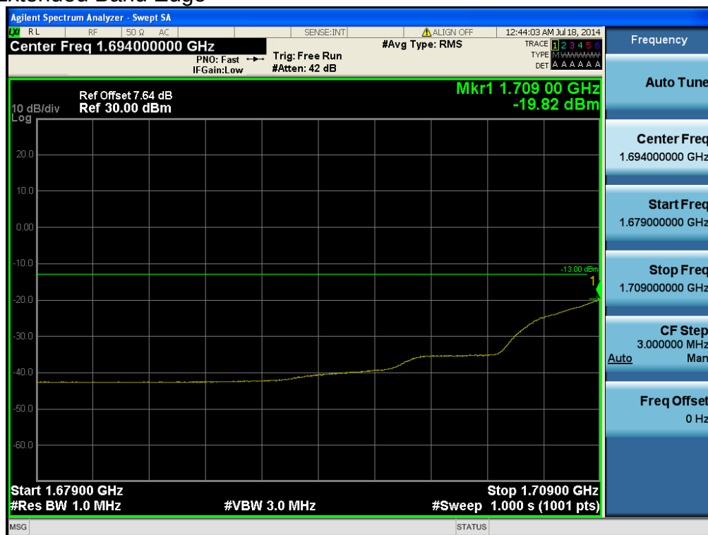
LTE Band 4 / 15MHz / QPSK - RB Offset/Size (0/36)
