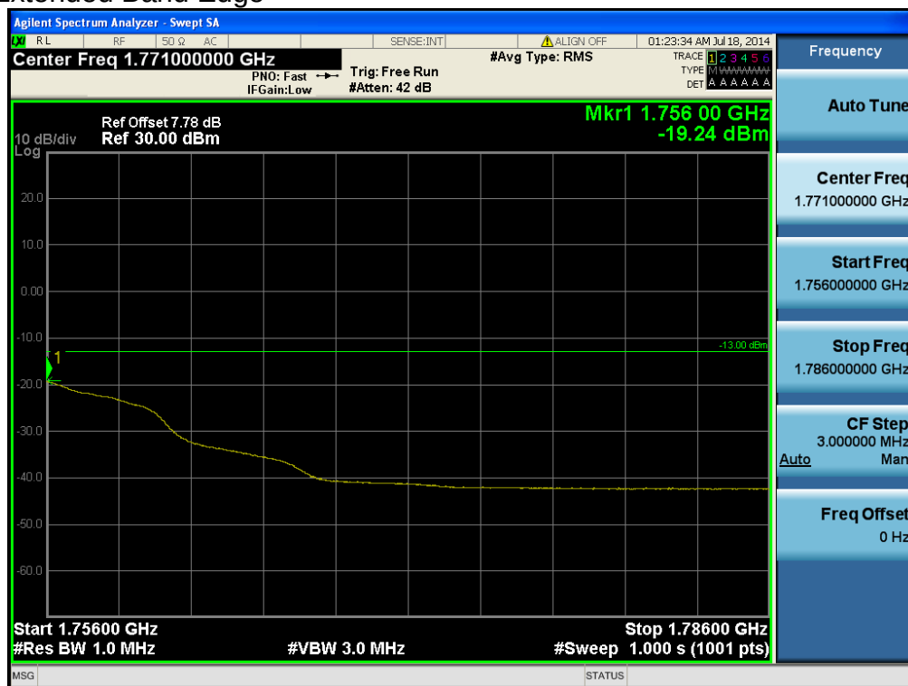
LTE Band 4 / 15MHz / QPSK - RB Offset/Size (39/36)
