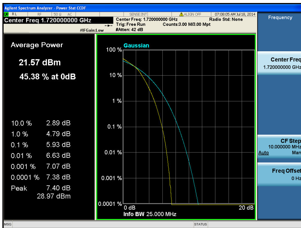
LTE Band 4 / 20MHz / 16QAM - RB Size 100
