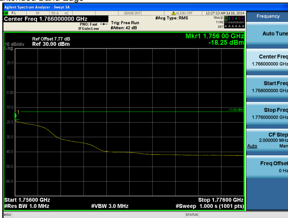
LTE Band 4 / 10MHz / QPSK - RB Offset/Size (25/25)
