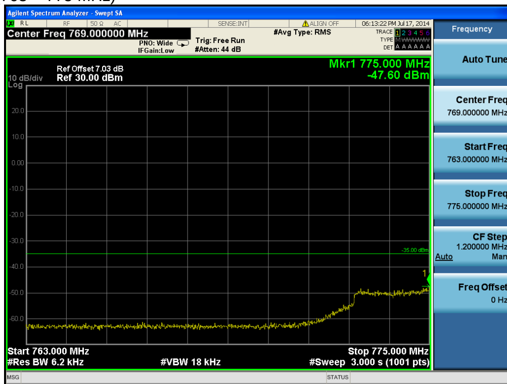
LTE Band 13 / 5MHz / QPSK - RB Offset/Size (0/25)
