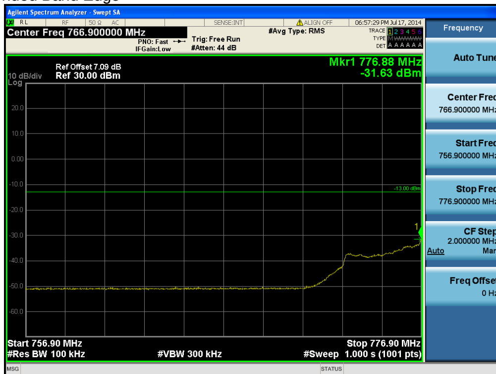
LTE Band 13 / 10MHz / QPSK - RB Offset/Size (0/25)
