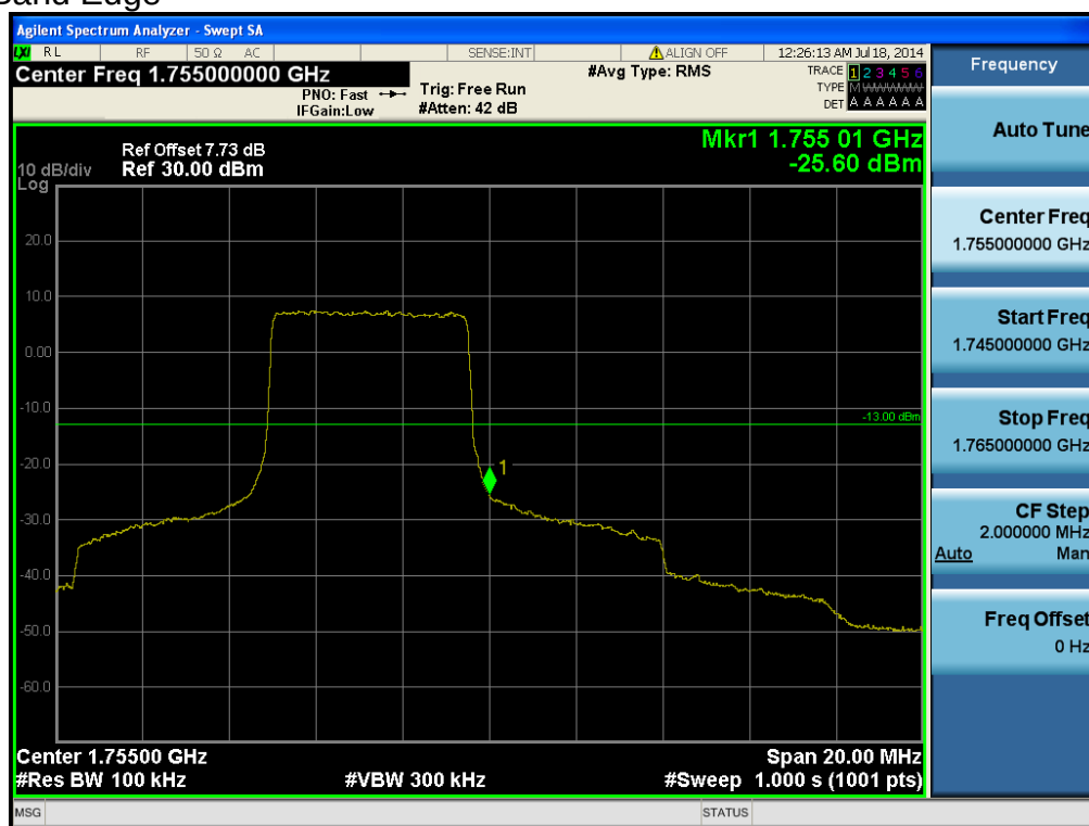
LTE Band 4 / 10MHz / QPSK - RB Offset/Size (25/25)
