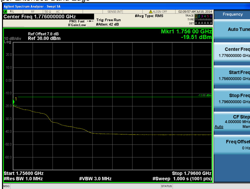
LTE Band 4 / 20MHz / QPSK - RB Offset/Size (50/50)
