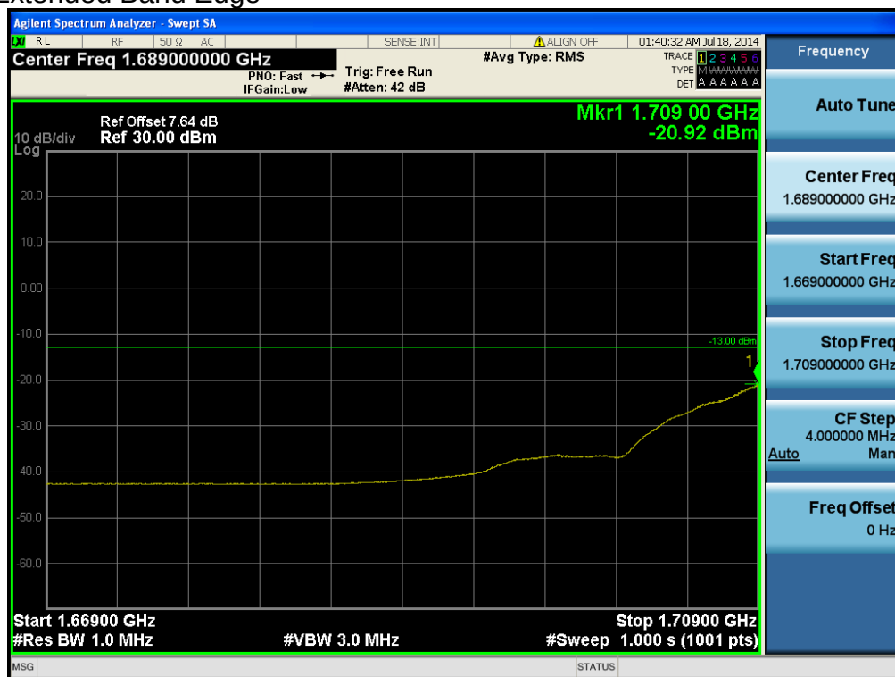
LTE Band 4 / 20MHz / QPSK - RB Offset/Size (0/50)
