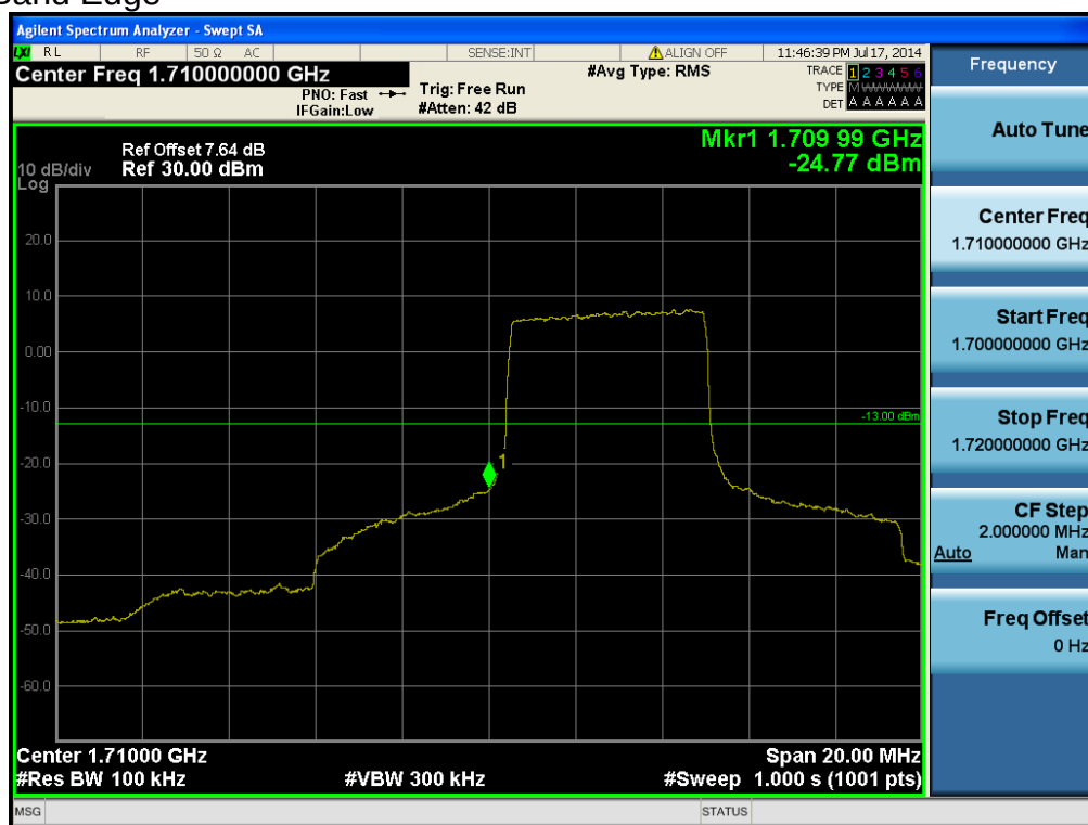
LTE Band 4 / 10MHz / QPSK - RB Offset/Size (0/25)
