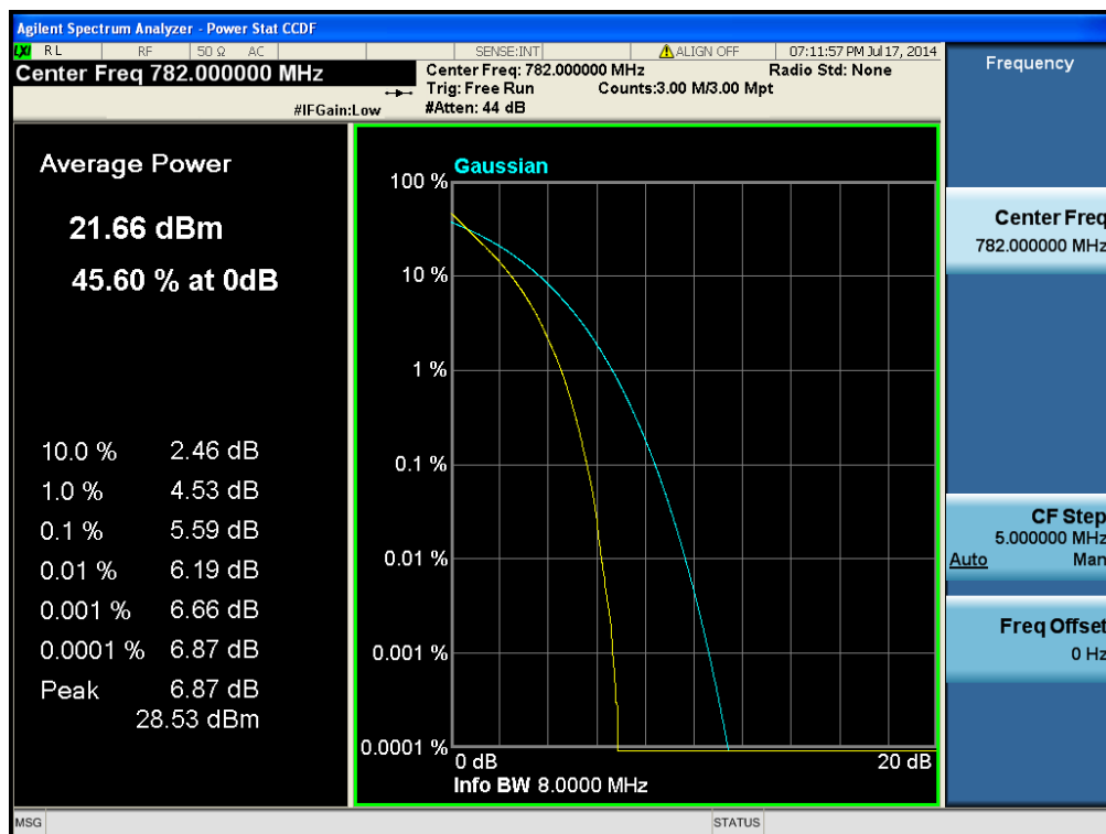
LTE Band 13 / 10MHz / QPSK - RB Size 50
