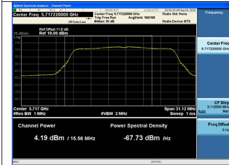
802.11n_HT20 UNII 2C Band Average Power CH.144
