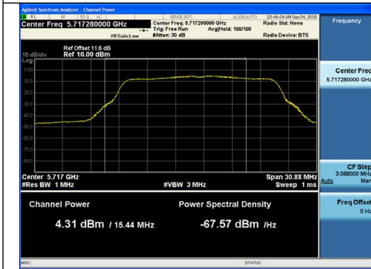
802.11n_HT20 UNII 2C Band Average Power CH.144
