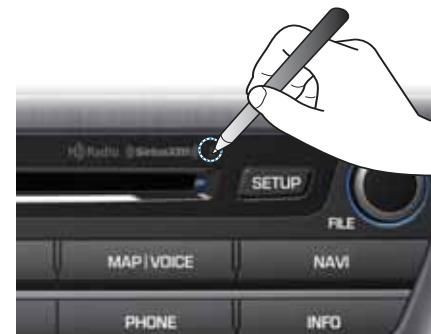
The System Reset function restores the system when it is not operating correctly. Press and hold the RESET key for a second or longer. (It is recommended that you press the RESET key using a tool, such as a pin or a clip.)
