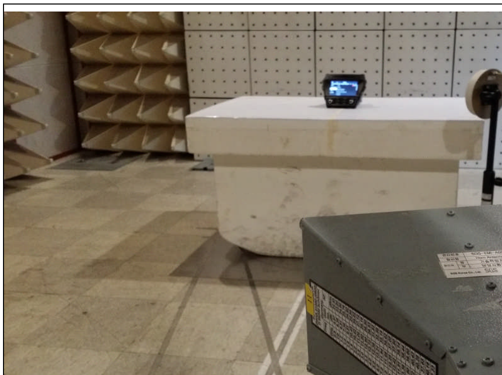
Photo of Field Strength & Spurious Emission Test(WLAN)
