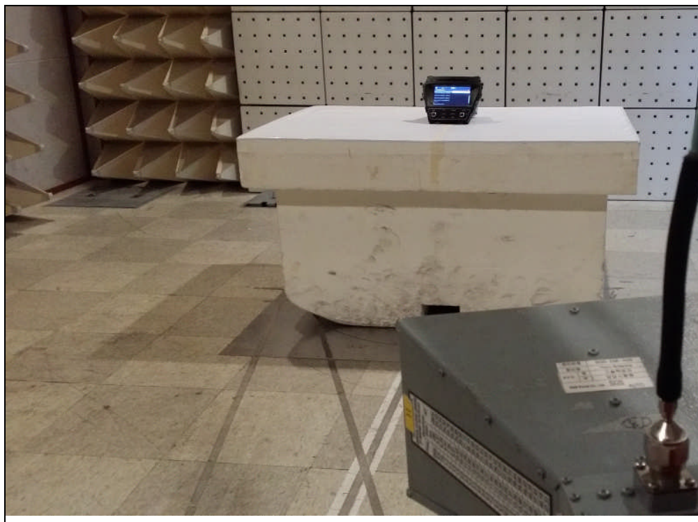
Photo of Field Strength & Spurious Emission Test(WLAN)
