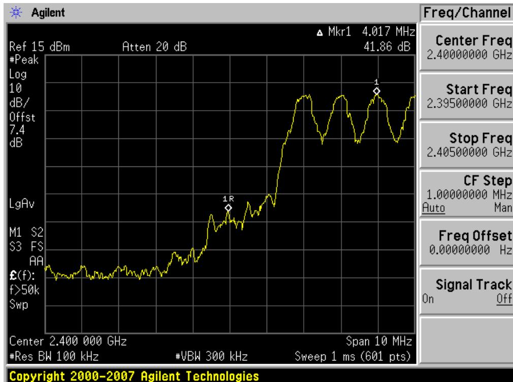
Test Plots with hopping (GFSK)
