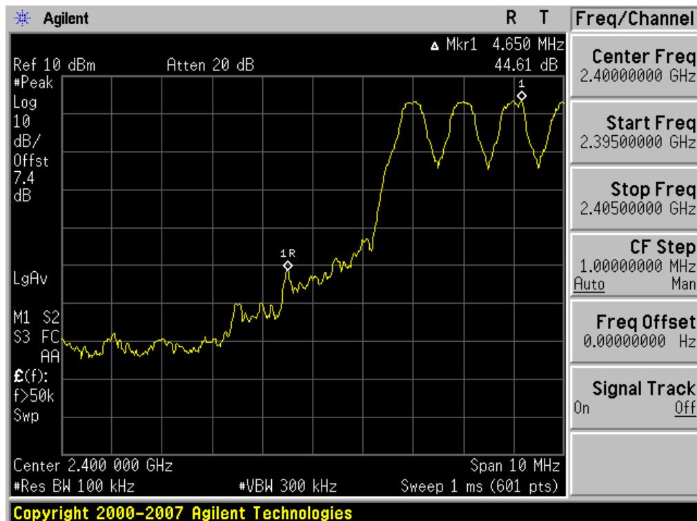
Test Plots with hopping (GFSK)
