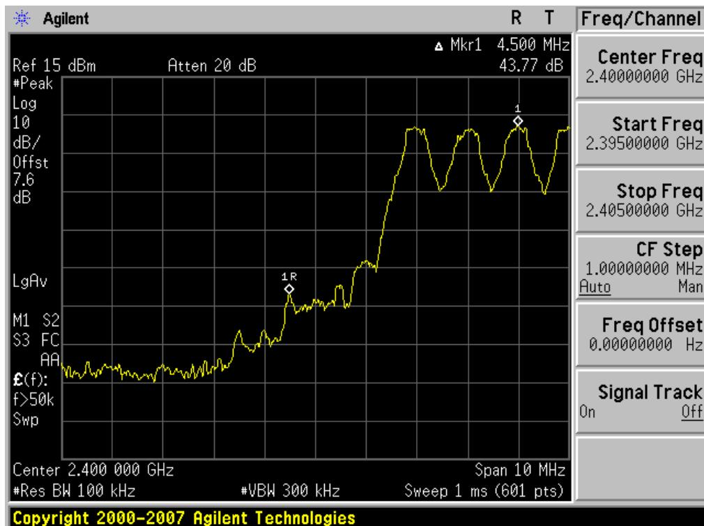
Test Plots with hopping (GFSK)
