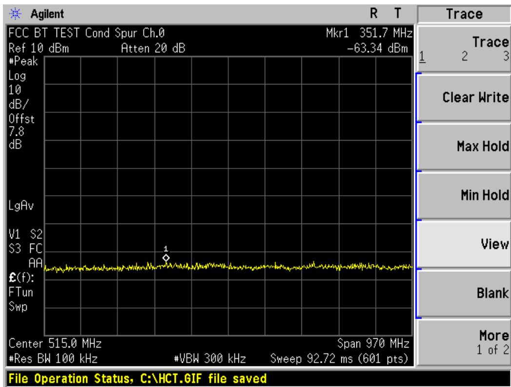
Test Plots (GFSK) - 30 MHz - 1 GHz (RBW:100 kHz, VBW: 300 kHz)
