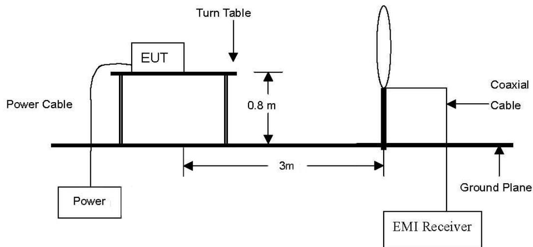
The diagram below shows the test setup that is utilized to make the measurements for emission from 30 GHz to 1 GHz Emissions.
