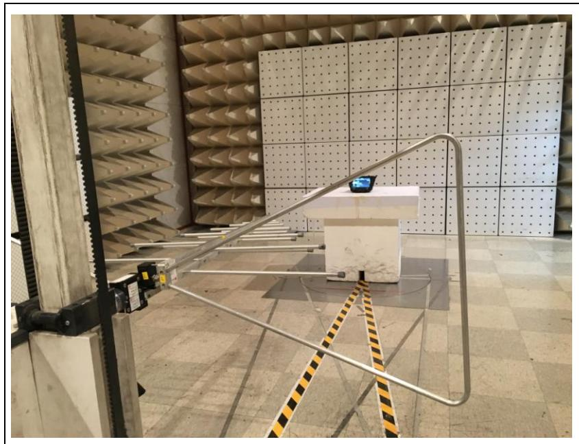
**3. Photo of Radiated Spurious Emission Test (Above 1 GHz)**
