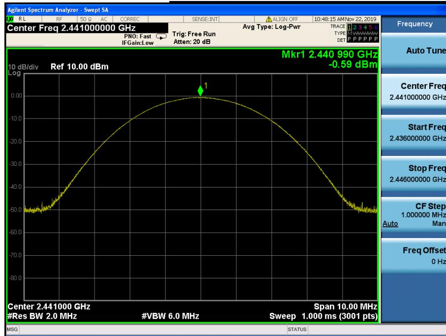
**Peak Output Power****Highest Channel & Modulation : 8DPSK**
