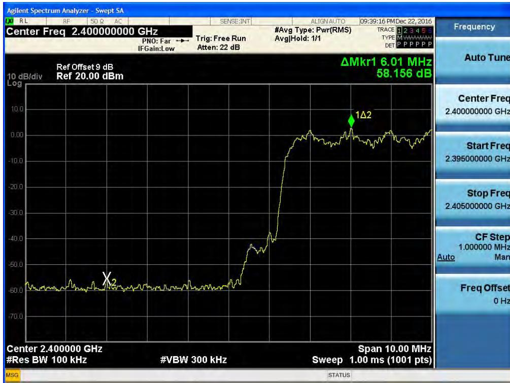
Test Plots with hopping (8DPSK)
