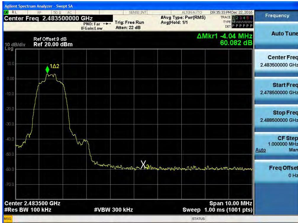
Test Plots with hopping (GFSK)
