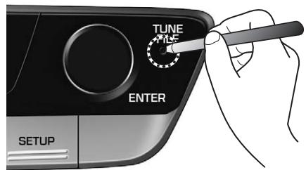
The System Reset function restores the system when it is not operating correctly. Press and hold the RESET key for a second or longer. (It is recommended that you press the RESET key using a tool, such as a pin or a clip.)
