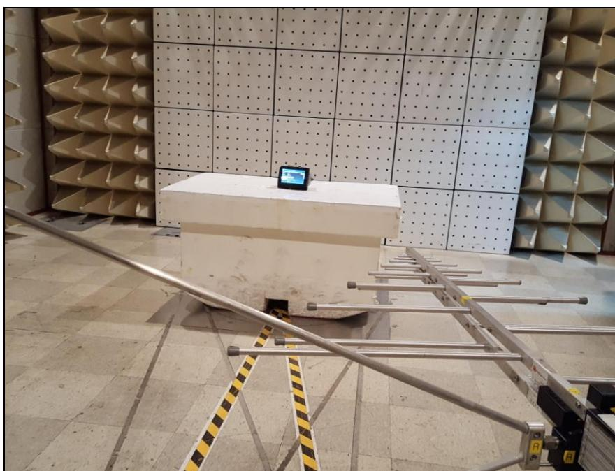
**3. Photo of Radiated Spurious Emission Test (Above 1 GHz)**
