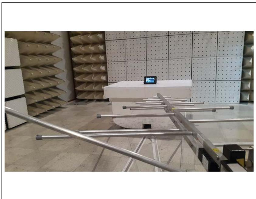
**3. Photo of Radiated Spurious Emission Test (Above 1 GHz)**
