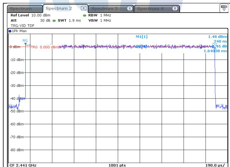
**3-DH5 (2 441 MHz)**
