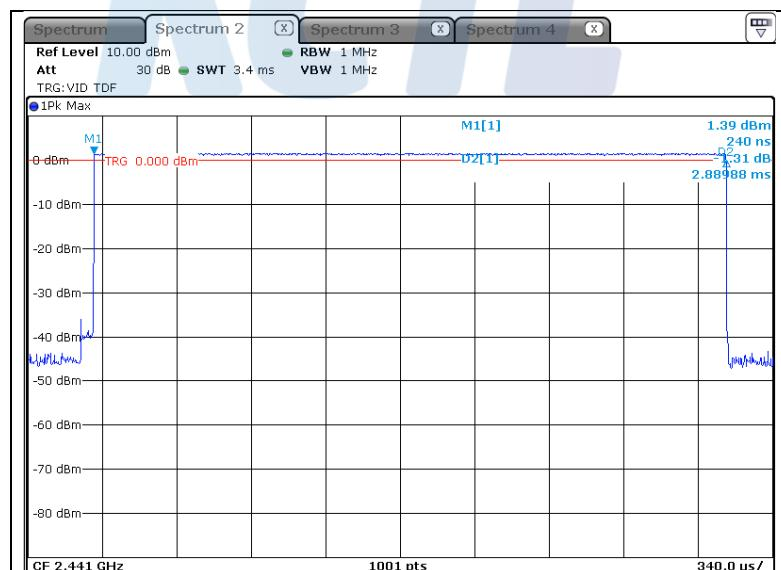
**- π/4DQPSK\_AFH mode****2-DH1 (2.441 MHz)**
