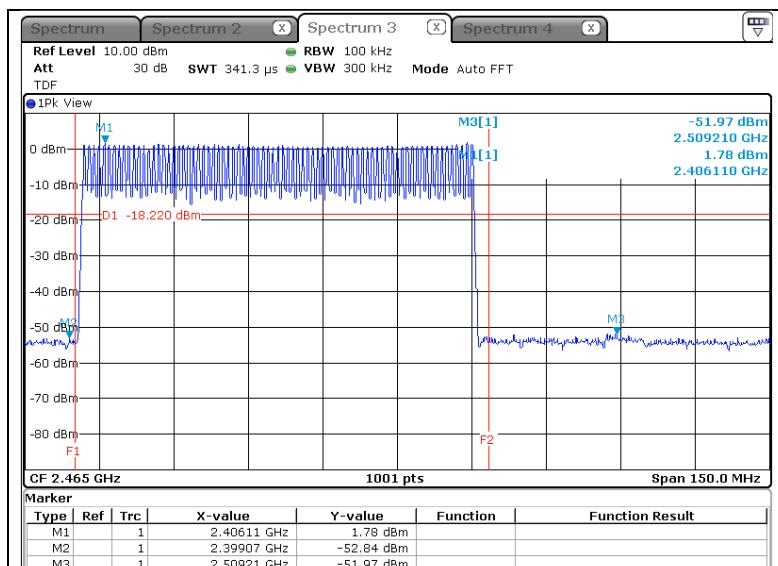
**- Result of 2 400.0 MHz - 2 483.5 MHz****- π/4DQPSK (Without hopping)****Lowest Channel (2 402 MHz)**
