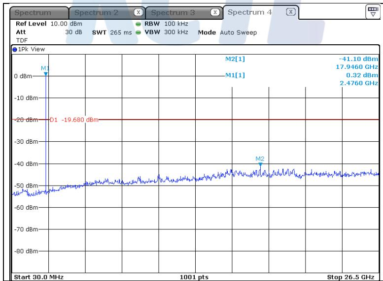
**- 8DPSK****Lowest Channel (2 402 MHz)**
