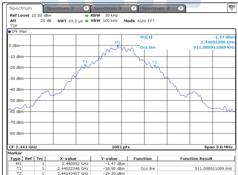
**Highest Channel (2 480 MHz)**
