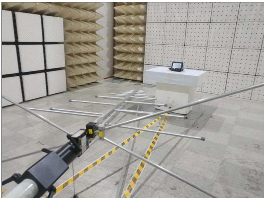
**3. Photo of Radiated Spurious Emission Test (Above 1 GHz)**
