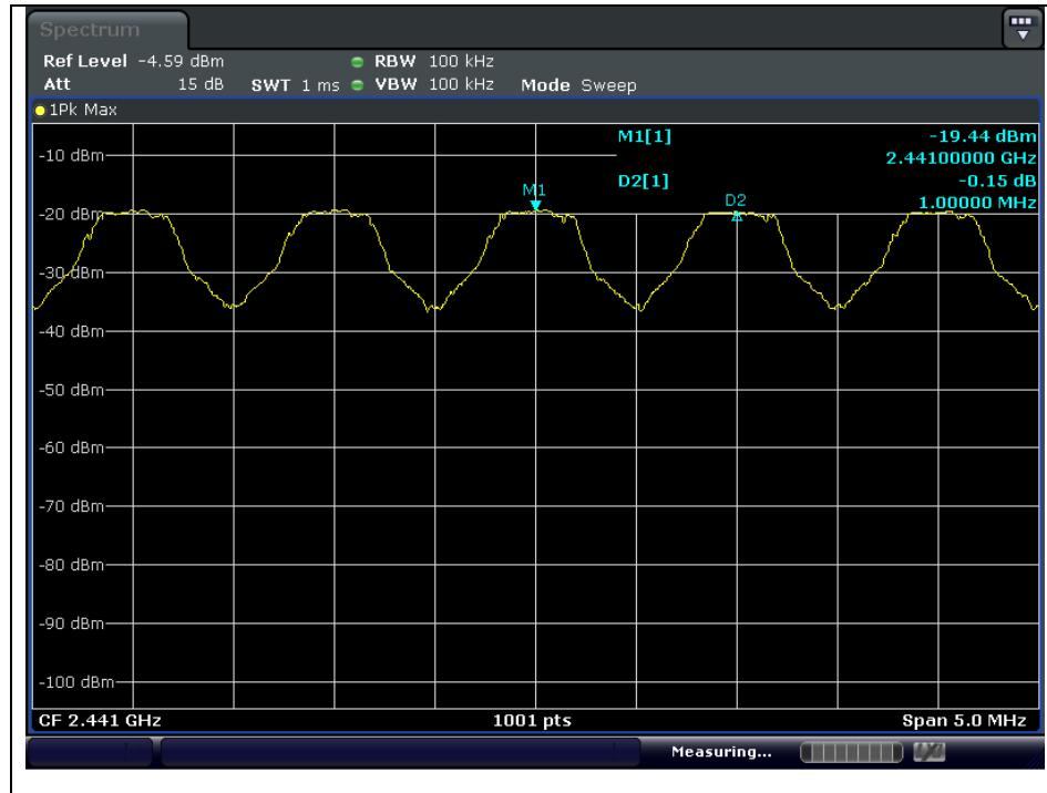
**Operating Mode: 8DPSK**
