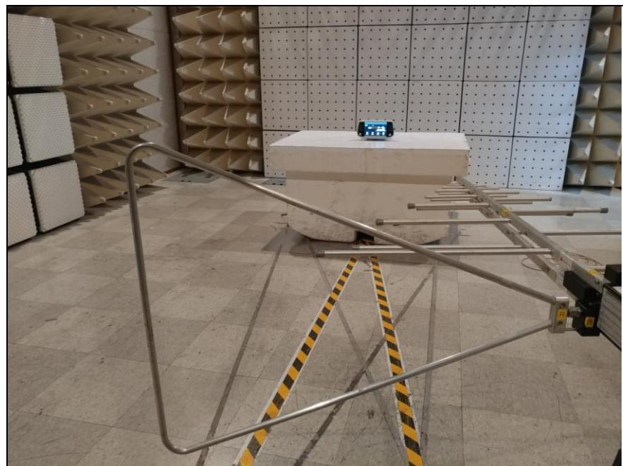
**2. Photo of Radiated Spurious Emission Test (Above 1 GHz)**
