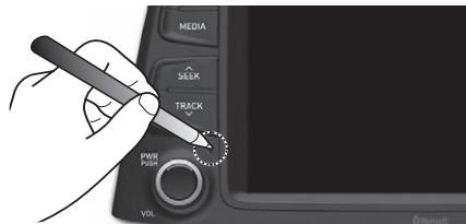
The System Reset function restores the system when it is not operating correctly. Press and hold the RESET key for a second or longer. (It is recommended that you press the RESET key using a tool, such as a pin or a clip.)
