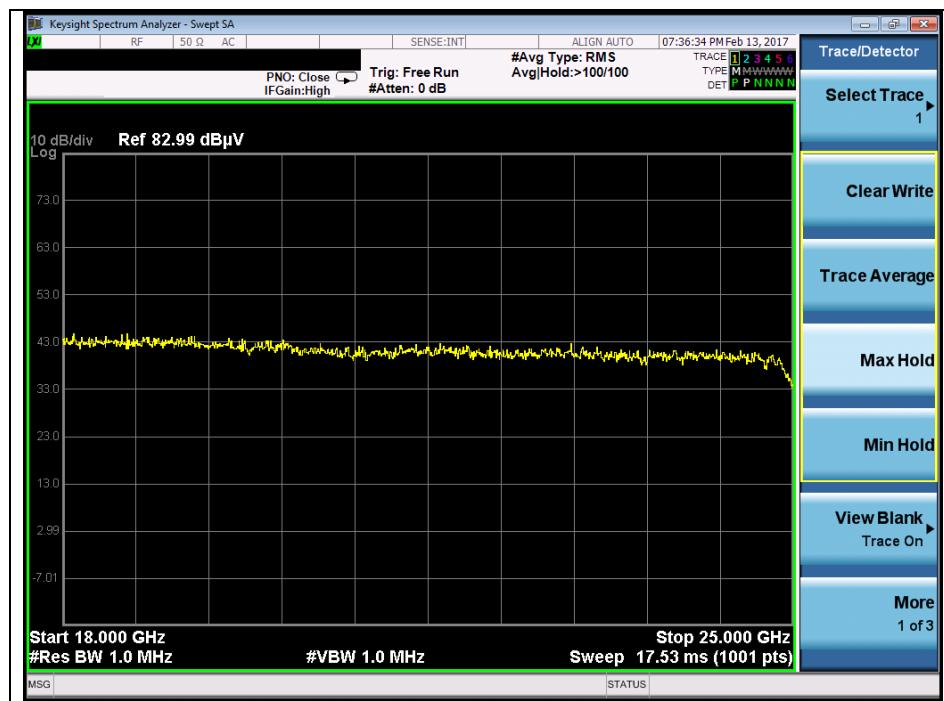
**Note:** Emission was scanned up to 25 GHz.
