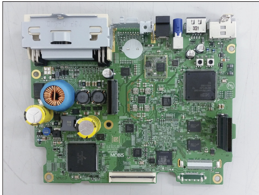
Top view of Main PCB
