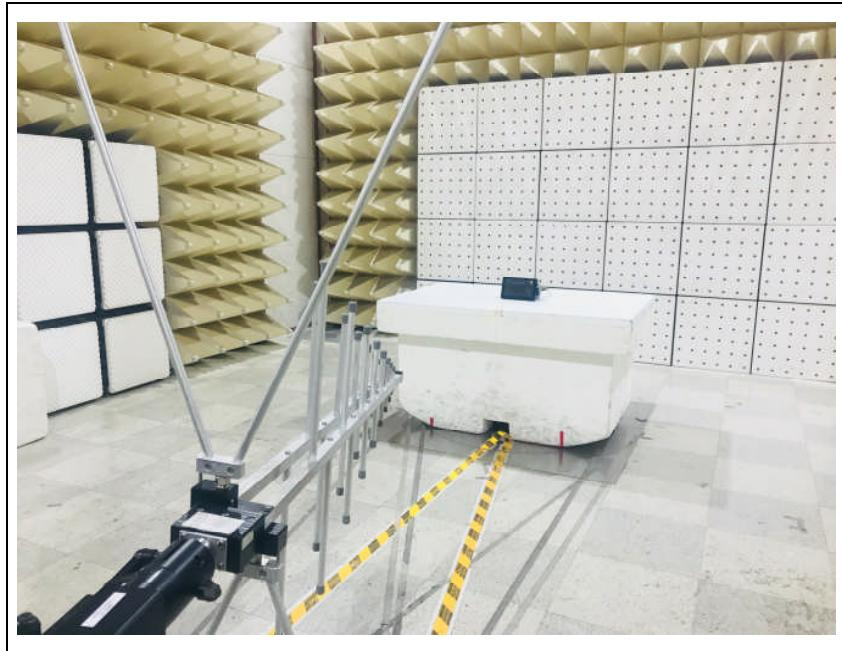
**3. Photo of Radiated Spurious Emission Test (Above 1 GHz)**
