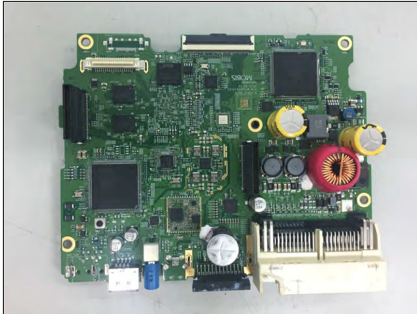
Bottom view of Main PCB1
